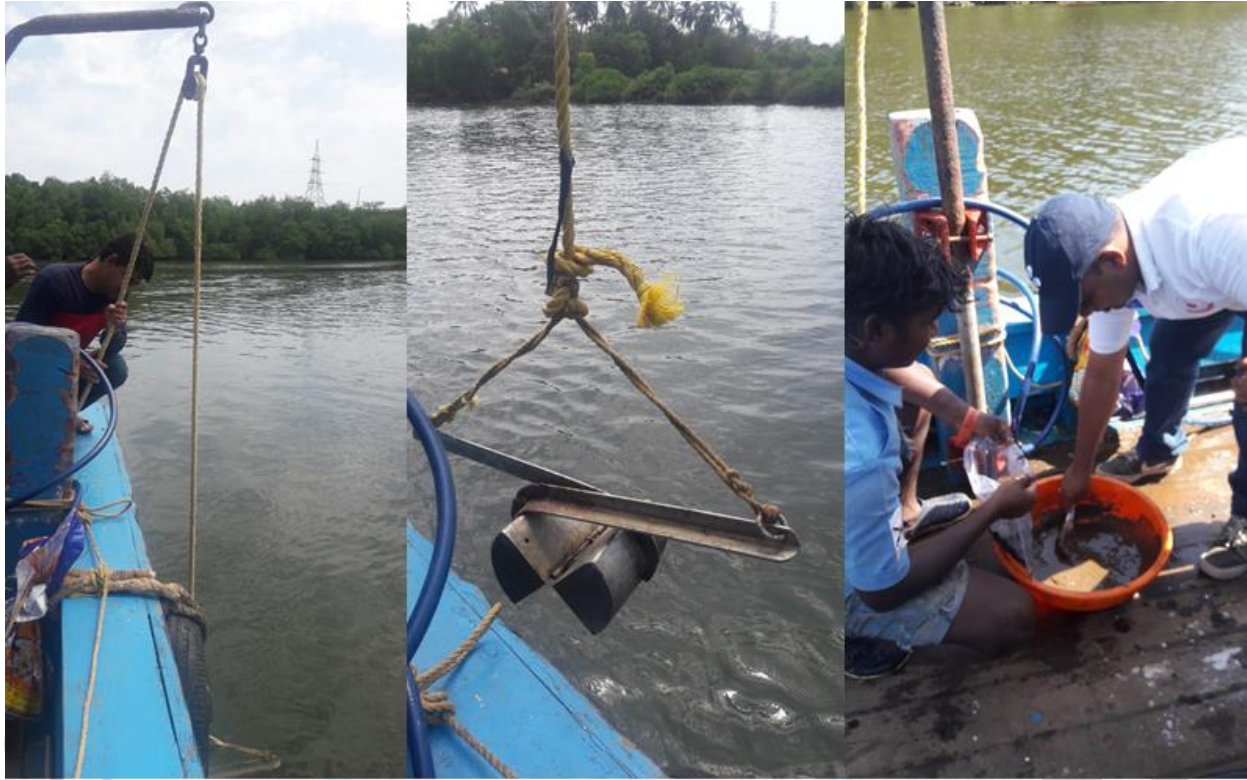
Figure 5. Sediment sample (hand grab sampler) photographs in Mandovi river
