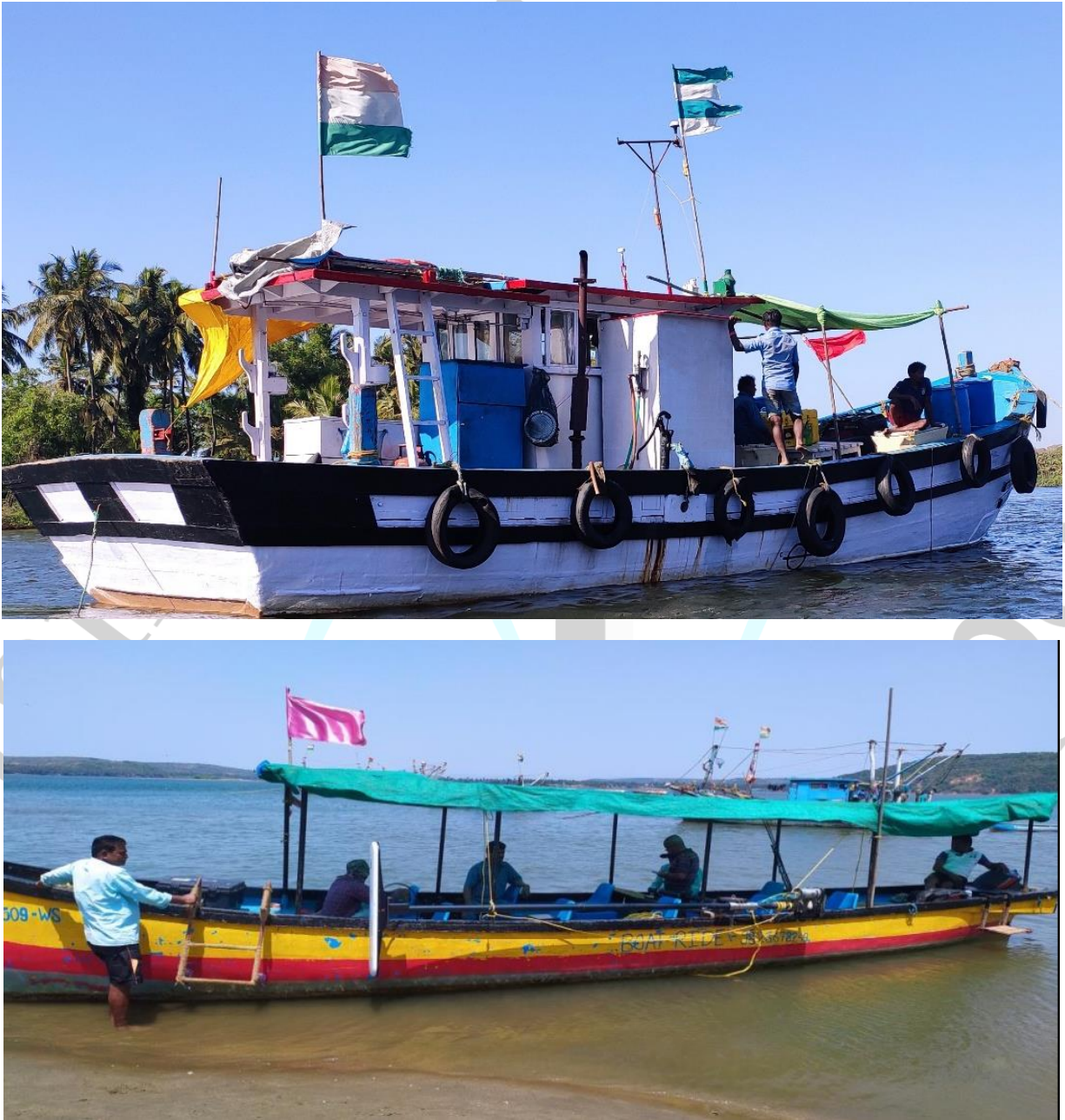
Figure 3. Boat deployed for survey for side scan sonar (SSS) imaging, single beam echosounder profiling, high resolution seismic (HRS squid) survey and geological sampling across the Mandovi river.
